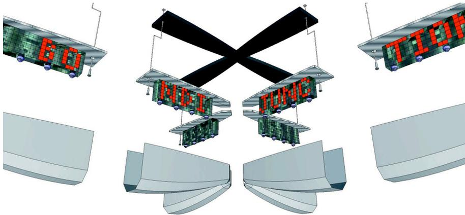
Figure 1. Exploded 3D view of lighting installation module © TBC
